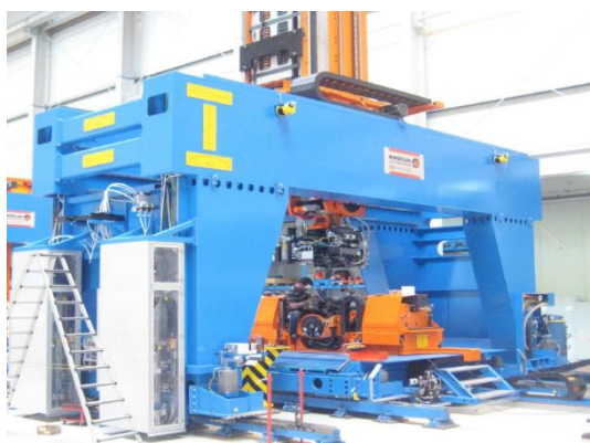
(a)德国宝捷的 MPAC (Multi-Panel Assembly Cell)
