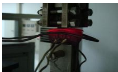
(c) XX9 涡轮叶片高温拉扭试验
