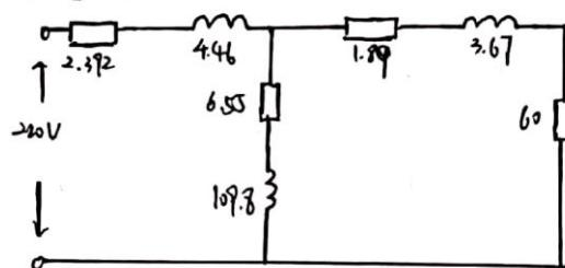
$$111. 空载输入阻抗 Z_0 = (r_1 + jx_{01}) + (t_m + jx_m) // (\frac{1}{S_N} r_2 + jx_{02}')$$
